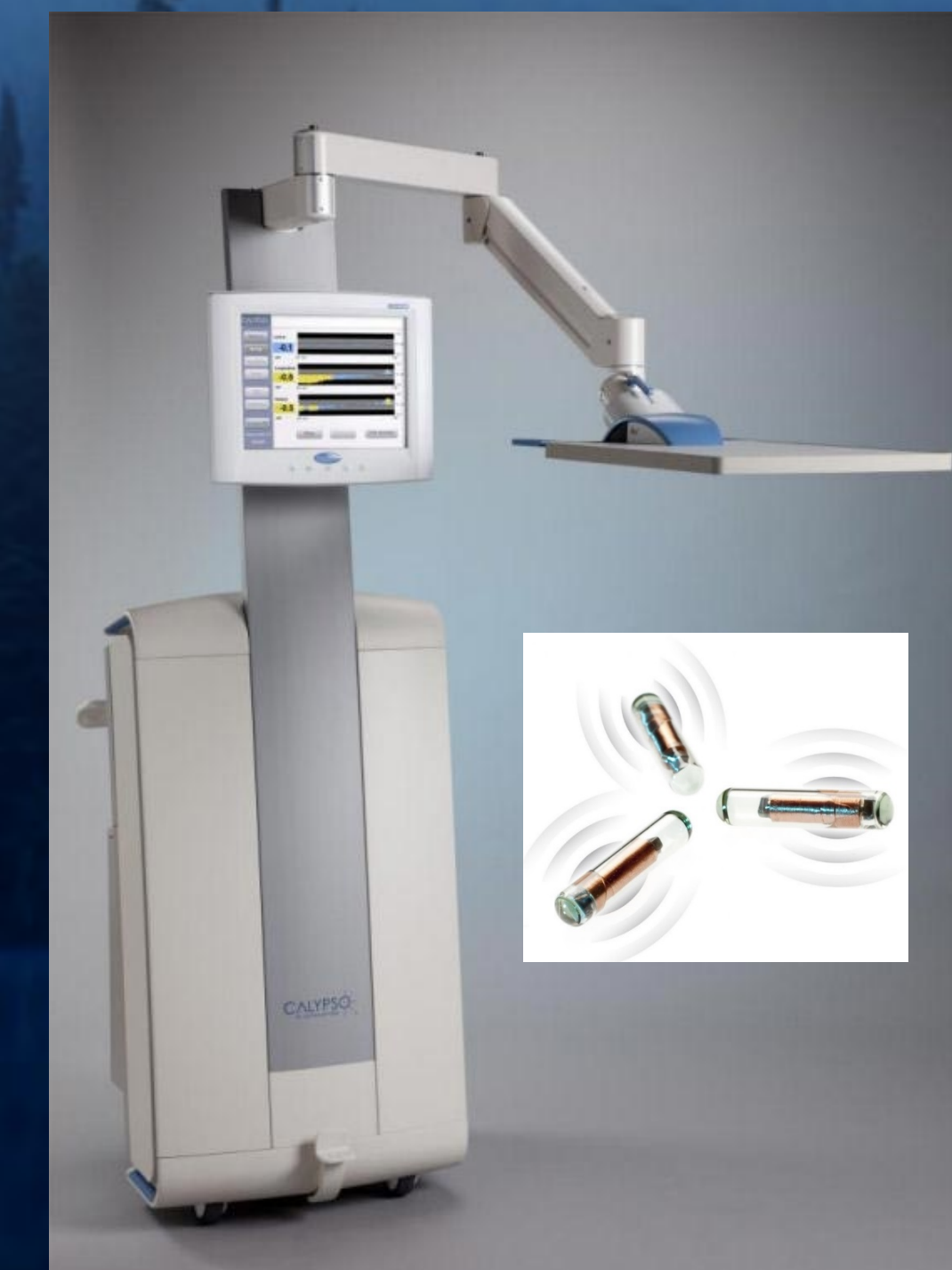
Calypso® System, for real-time tumor motion tracking, developed in Seattle and acquired by Varian in 2011
